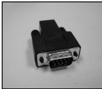
Figure 8. Supplied interlock defeat connector.
