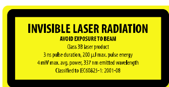
Figure 4. Laser information label, located on back panel.
